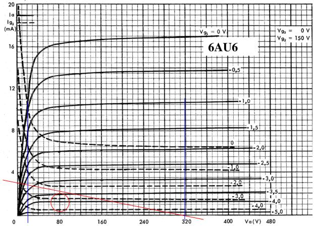
Modified amp with 500k pickup volume pot after 6AU6, loads down gain a bit more.
